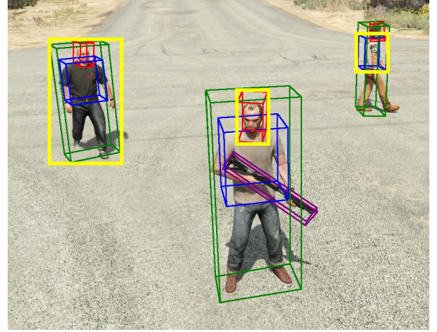
Fig. 4. Bounding box estimation: oversized approximation with respect to on-screen projections. With the available API, the hooked virtual engine is able to provide the bounding boxes of individual 3D meshes, overestimated due to collision proxy expansion for animations. Not being able to access the original 3D geometry and the current animation frame, our best strategy is to project on-screen the eight corners of the 3D bounding box, and then take their containing minimum rectangle as our best annotation.
